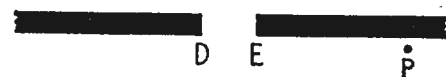
Fig. 4. Although opposite sides, D and E, of this wider opening are in phase as regards the original source of waves, their wavelets reach P out of phase, tending to cancel one another and reduce diffraction.
